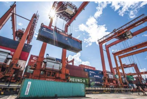
The terminal operators frequently upgrade their equipment and systems to enhance efficiency and to offer a better operation environment. Apart from electric Rubber-Tyred Gantry Cranes (RTGCs) and hybrid machines, Container Terminal 9 North launched a remote-controlled RTGCs and automated container stacking system in early 2018. This represents a new era of terminal operation, not only to raise operational efficiency and productivity, but also to strengthen competitiveness of the terminals.
